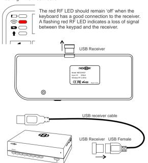
The range of the keyboard can be effected by metal content so we suggest that the USB receiver be placed away from the player or any other metal object. Unclip the USB receiver from the keyboard and plug in into the USB Female connector. Plug the male USB into one of the USB host ports on the Mede8er. Position the USB Receiver as far away from the player as possible with clear sight to the keyboard.
